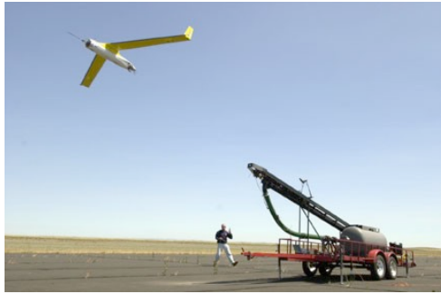
Fig. 1. A sample Real-time Java application: the first integrated real-time Java system on the ScanEagle Unmanned Aerial Vehicle [9]. The flight hardware/software was an Embedded Planet PowerPC 8260 processor running at 300MHz with 256 MB SDRAM and 32 MB FLASH. The operating system is Embedded Linux.
