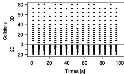
Figure 6. Collisions in COL workload. The upper graph shows 3D collisions and the lower the number of 2D collisions.
