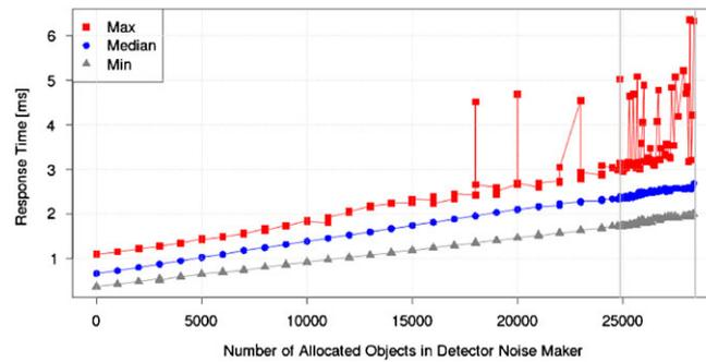
Figure 14. Sample stress test: response time for an increasing amount of allocation noise on RTS.
