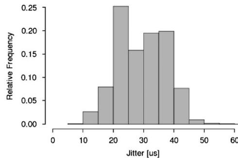
Figure 13. Relative frequency histogram of release jitter.
