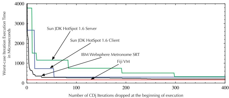
Figure 15. Start-up costs. The Y-axis is the worst case observed execution time, whereas the X-axis shows iterations dropped from the 10 000 performed for each VM. The initial iterations are dominated by the just-in-time compiler. If roughly 300 or more iterations are dropped, the worst case is dominated by garbage collection.
