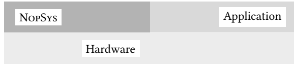
Figure 1. High-level architecture: NopSys is a library to run applications on the bare metal.
